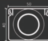
Insulated Drain Pipe
